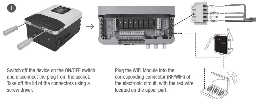
Switch off the device on the ON/OFF switch and disconnect the plug from the socket. Take off the lid of the connectors using a screw driver.
